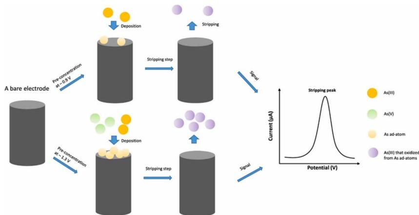
Fig. 16 The total arsenic concentration measured by deposition at  $-1.3$  V while the  $\text{As(III)}$  measured at  $-0.9$  V on gold macroelectrodes based on the underpotential deposition (UPD) of As ad-atoms<sup>131</sup> (reprinted from ref. 131; Copyright (2022), with permission from Elsevier).
