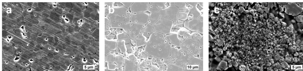
Fig. 4 SEM micrographs of samples sintered under different conditions: (a) flash-sintered sample from micropowder at 150 V cm<sup>-1</sup> and 15 mA mm<sup>-2</sup>; (b) conventionally-sintered sample from nanopowder; (c) flash-sintered sample from nanopowder at 150 V cm<sup>-1</sup> and 15 mA mm<sup>-2</sup>.
