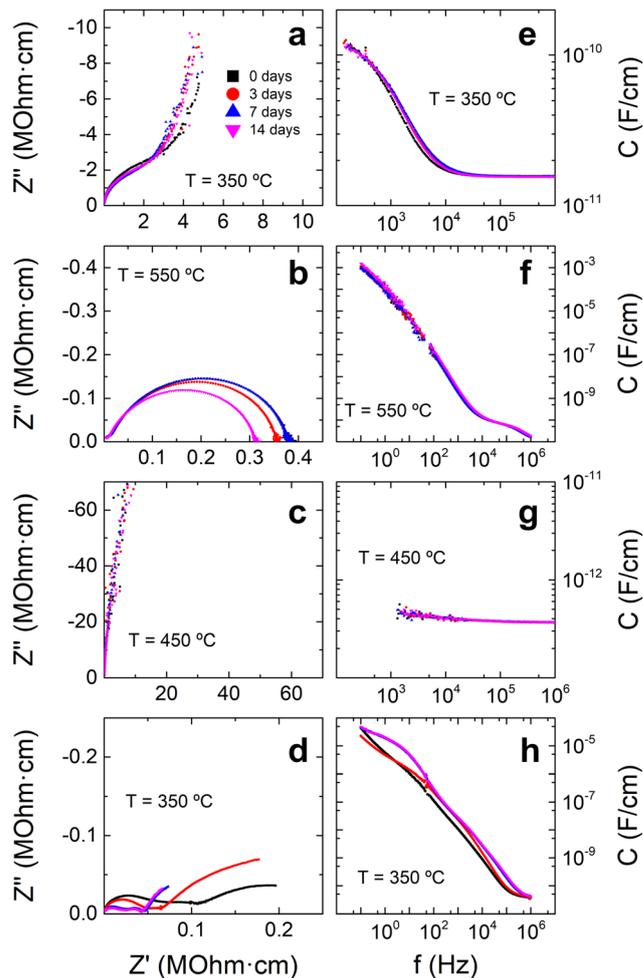
Fig. 2 Time evolution of (a)–(d) Nyquist plots and (e)–(h) capacitance versus frequency response of samples sintered under different conditions: (a), (b), (e) and (f) flash-sintered from micropowder; (c) and (g) conventionally-sintered from nanopowder; (d) and (h) flash-sintered from nanopowder. Samples were flash-sintered at  $150 \text{ V cm}^{-2}$  and  $15 \text{ mA mm}^{-2}$  with a dwell time of 10 min.
