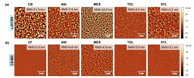
Atomic force microscopy (AFM) images of (a) o-IDTBR and (b) L8-BO films processed using different solvents
