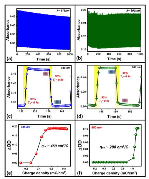
Fig. 4 (a) In situ bias-dependent multiple switching cycles of the device between ON and OFF states in the voltage window (±1.5 V) in the visible and infrared (IR) wavelength region in (b) and (c) single switching cycle at 515 nm wavelength, (d) response time of the device in the same fixed voltage window at 800 nm wavelength, and the corresponding estimated coloration efficiencies of the device in (e) and (f).
