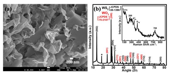
Fig. 1 (a) FESEM micrograph; (b) XRD pattern of WS<sub>2</sub>/WO<sub>3</sub> nanoflakes along with their Raman spectra (inset).
