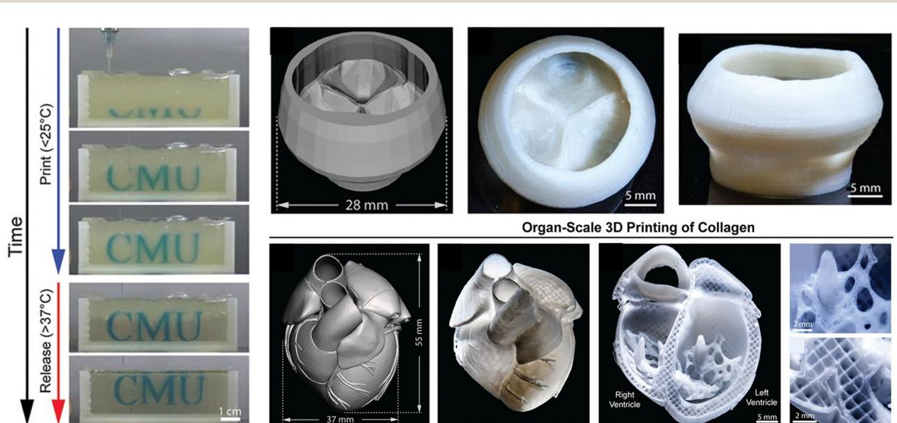
Fig. 11 A thermo-reversible gelatin microgel as the supporting bath for FRESH printing. Reproduced with permission from ref. 138. Copyright 2019 The Authors.
