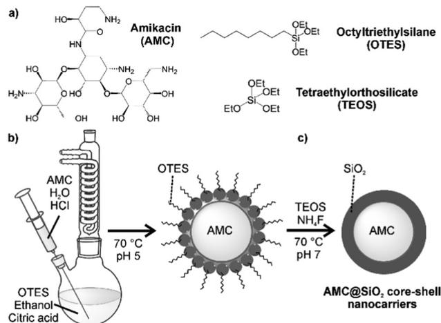
Fig. 1 Schematic illustration of the synthesis of AMC@SiO<sub>2</sub> core@shell nanocarriers: (a) starting materials, (b) nucleation via a solvent–antisolvent approach, (c) densification and thickening of silica shell.
