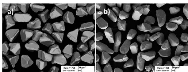
Fig. 6 SEM images of (Cu<sub>1-x</sub>Ag<sub>x</sub>)<sub>1.85</sub>(Zn<sub>0.8</sub>Cd<sub>0.2</sub>)<sub>1.1</sub>SnS<sub>4</sub> monograin powder crystals: (a) *x* = 0 and (b) *x* = 0.15. Reproduced from ref. 28 with permission from the Royal Society of Chemistry, Copyright 2019.
