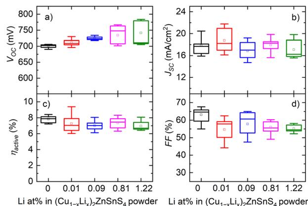
Fig. 11 Box-plot diagram of CZTS solar cell parameters (a) open circuit voltage ( $V_{\text{OC}}$ ), (b) current density ( $J_{\text{SC}}$ ), (c) efficiency ( $\eta_{\text{active}}$ ) and (d) fill factor (FF) with different Li concentrations in the CZTS powder. Reproduced from ref. 32 with permission from Elsevier B.V., Copyright 2023.
