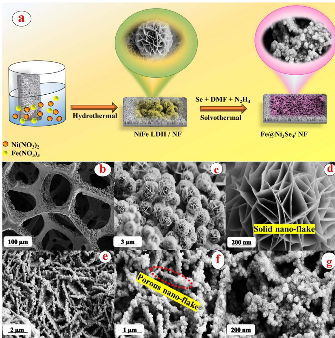
Fig. 1 (a) Schematic diagram for the overall design strategy adopted for the synthesis of  $\text{Fe@Ni}_3\text{Se}_4$  from NiFe-LDH; (b–d) low- to high-magnification FE-SEM images for pristine NiFe-LDH grown over metallic nickel foam. (e–g) Low to high magnification FE-SEM images of the sheet-like Fe-doped  $\text{Ni}_3\text{Se}_4$  with a microporous structure.
