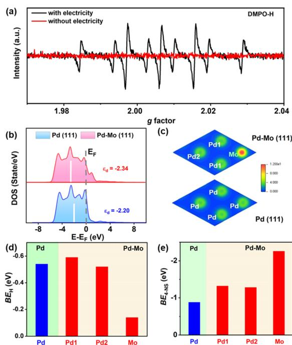
Fig. 4 (a) Quasi *in situ* EPR trapping of hydrogen radicals over Pd–Mo metallene. (b) PDOS for the d band of Pd and PdMo, and (c) electron density difference with Pd (111) and Pd–Mo (111). (d)  $BE_H$  and (e)  $BE_{4-NS}$  on Pd (111) and Pd–Mo (111).
