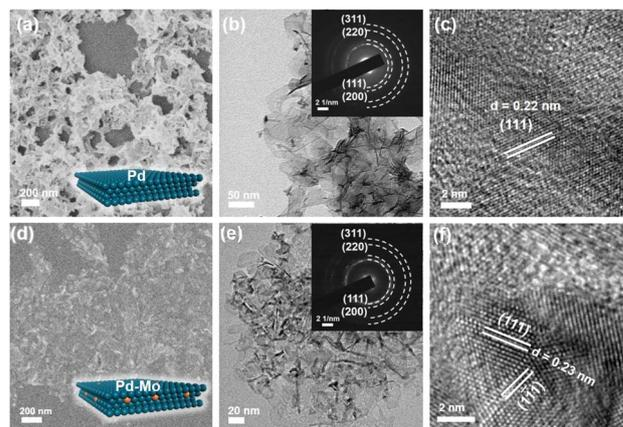
Fig. 1 (a and d) SEM, (b and e) TEM, and (c and f) HR-TEM images of (a–c) Pd and (d–f) Pd–Mo metallenes. Insets of (b) and (e) display the SAED images.
