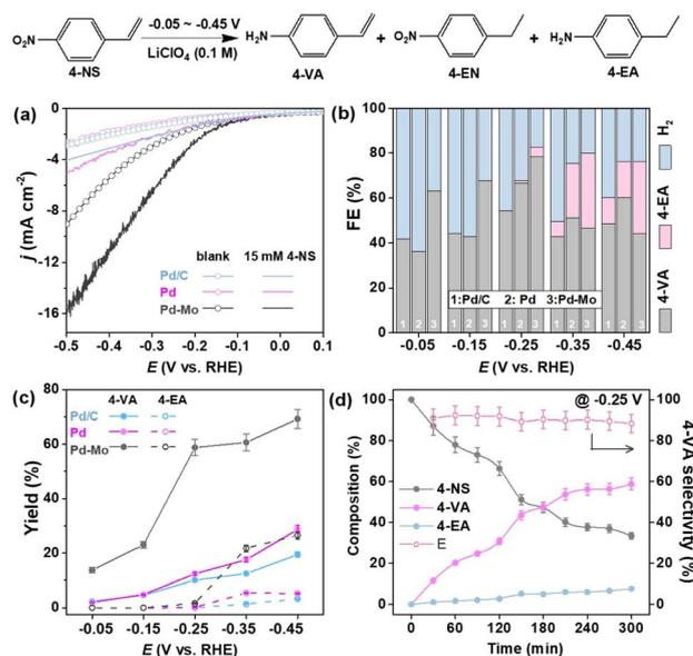
Fig. 3 ECH performance of 4-NS over Pd-based metallenes. (a) Polarization curves of Pd–Mo and Pd metallenes and commercial Pd/C in 0.1 M LiClO<sub>4</sub> with and without 15 mM of 4-NS at a scan rate of 10 mV s<sup>-1</sup>. (b) FEs and (c) yields of products for the ECH of 4-NS over Pd-based metallenes and commercial Pd/C in a wide potential range of –0.05 to –0.45 V vs. RHE (4-NS: 15 mM, reaction time: 5 h). (d) Time curves of 4-NS, 4-VA and 4-EA on the Pd–Mo metallene at –0.25 V vs. RHE.
