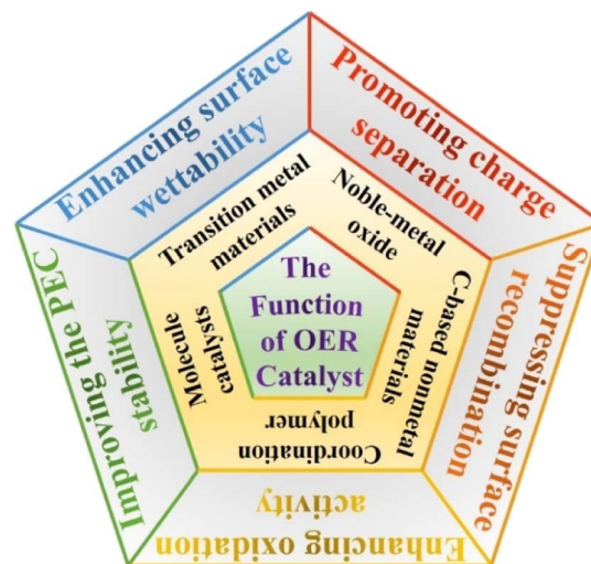
Fig. 2 The schematic illustration of the function of OER catalysts in PEC water splitting.
