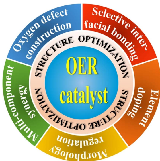
Fig. 3 The summary of design strategies for further enhancing the OER catalyst activity.
