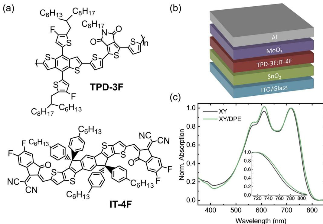
**Fig. 1** (a) Chemical structures of the polymer donor TPD-3F and the non-fullerene acceptor IT-4F. (b) Schematic of the device structure used in this work. (c) Absorption spectra of TPD-3F:IT-4F blend films cast from *o*-xylene without additive and with 3 wt% of DPE. The inset shows a zoom-in of the absorption onset.
