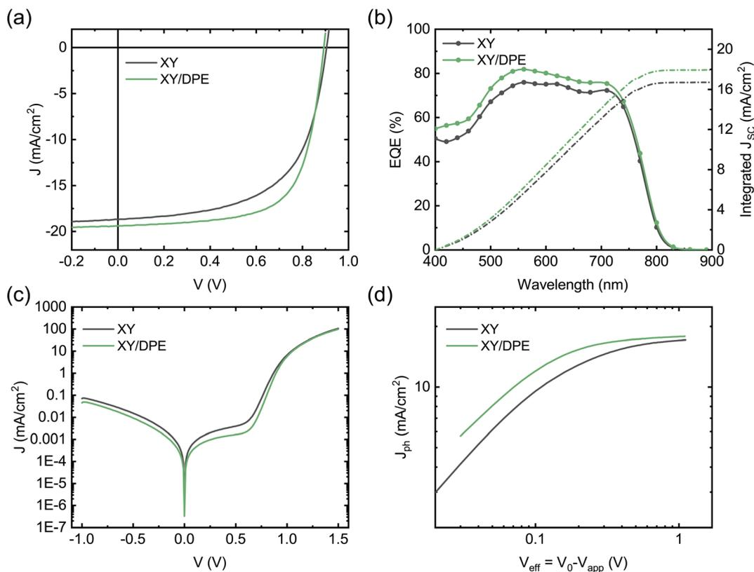
Fig. 2 Electrical characteristics of optimized solar cells, fabricated by spin coating from a *o*-xylene solution without additive and with 3 wt% of DPE: (a)  $J$ - $V$  curves under illumination (AM 1.5,  $100 \text{ mW cm}^{-2}$ ); (b) EQE spectra and integrated  $J_{sc}$ ; (c)  $J$ - $V$  curves in dark condition; (d)  $J_{ph}$  as a function of  $V_{eff}$ .
