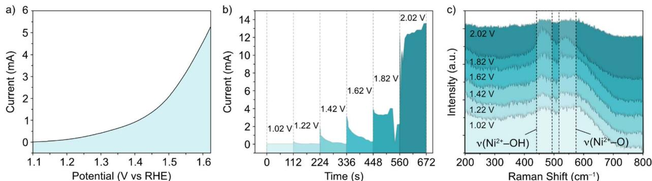
Fig. 2 (a) Polarization curve, (b) successive chronoamperometry curves at potentials between 1.02–2.02 V vs. RHE, and (c) *in situ* Raman spectra in the selected wavenumber range for NiFe LDH on an indium tin oxide-coated glass substrate, compatible with the *in situ* electrochemical setup.
