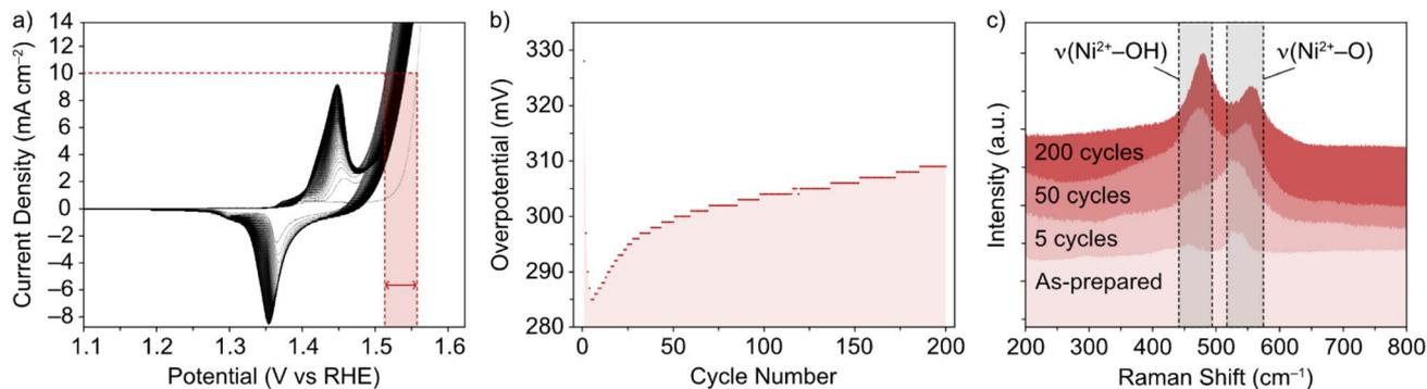
Fig. 1 (a) CV of NiFe LDH loaded on nickel foam in 1 M KOH, and (b) resulting overpotential values ( $\pm 7$  mV) for OER as a function of cycle number, through 200 cycles. (c) Corresponding *ex situ* Raman spectra in the selected wavenumber range 200–800  $\text{cm}^{-1}$  for NiFe LDH on Ni foam, (from bottom) for the as-prepared catalyst, and after 5, 50 and 200 CV cycles between 1–1.6 V vs. RHE at 5  $\text{mV s}^{-1}$ .
