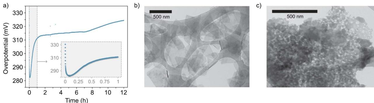
Fig. 3 (a) Chronopotentiometry curve of the catalyst at  $10 \text{ mA cm}^{-2}$  for 12 hours (inset, close-up view of the first hour). (b) and (c) Representative areas of the NiFe LDH samples before and after 50 OER cycles (ESI Fig. S4<sup>†</sup>), respectively, imaged with STEM.
