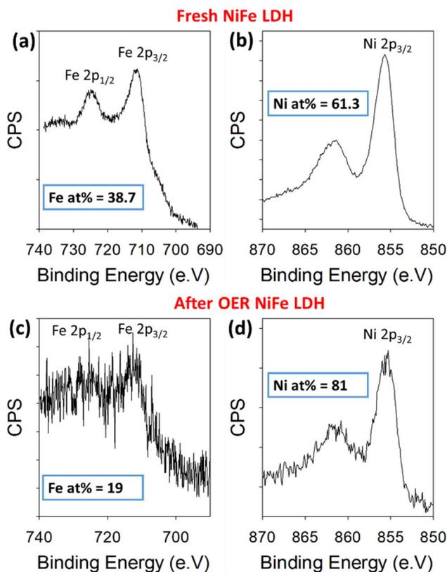
Fig. 4 Binding energy XPS spectra for Fe 2p and Ni 2p core levels before cycling (a and b) and after 50 cycles (c and d) within a NiFe LDH catalyst on Au/Ti/SiO<sub>2</sub>/Si.
