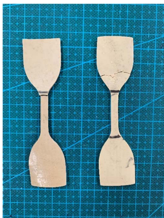
Fig. 33 Dumbbell test piece of (Left) natural rubber and (Right) natural rubber nano cellulose composite material. 160
