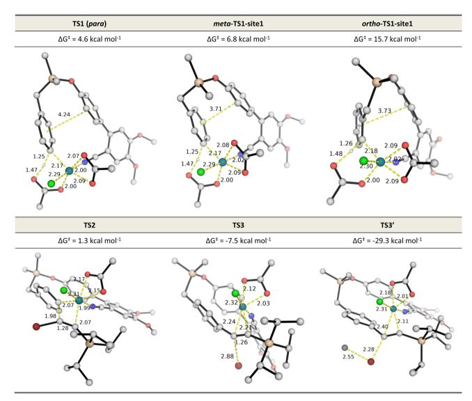
Fig. 2 DFT optimized TS structures for the C-H activation at different arene sites (TS1s), migratory insertion (TS2) and  $\beta$ -bromide elimination without (TS3) and with (TS3') silver ion participation. All Gibbs energies are taken with INT1 as zero reference. See Fig. S5† for C-H activation TSs of all possible sites.
