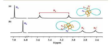
Fig. 3 Comparison of the  $^1$ H NMR spectra (600 MHz, CDCl<sub>3</sub>, 298 K) of (a) bis-po-CC and (b) bis-pm-TC.
