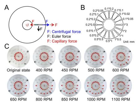
Fig. 1 Schematic and test of the superhydrophobic valve. (A) The force analysis of fluid in the CD microfluidic chip. (B) The structure of the CD microfluidic chip containing microchannels of different sizes. (C) Flow stage of the sample liquid in the chip with increasing rotation speed and time. The scale bar is 1 cm.
