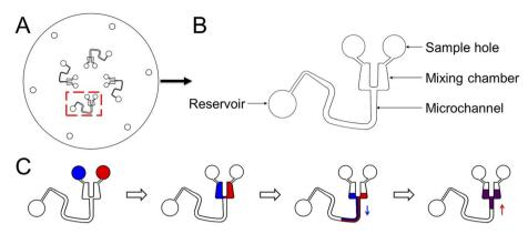
Fig. 2 The design of the CD microfluidic chip and illustration of the mixing process. (A) Illustration of the whole CD chip. (B) Illustration of one of the channels for mixing liquid. (C) The reciprocating motion of liquid in the modified microchannel. The blue arrow represents the direction of centrifugal force. The red arrow represents the direction of capillary force.
