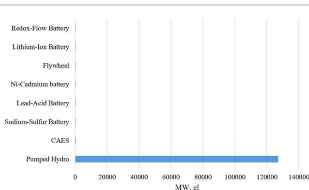
Fig. 1 Worldwide energy storage systems for electricity production.<sup>35</sup>
