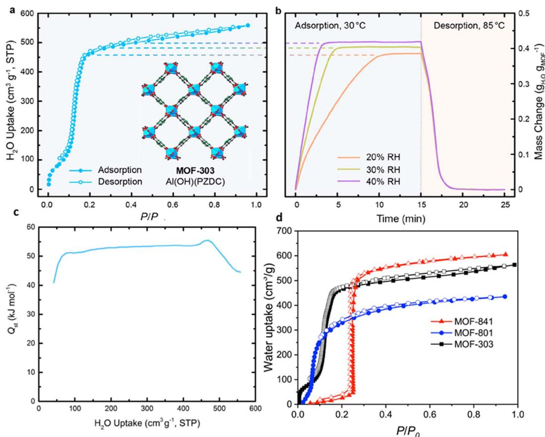
Fig. 36 Water adsorption properties of MOF-303. (a) Water adsorption isotherm at 30 °C. (b) Water vapor adsorption & desorption behavior. (c) Isostatic heat of adsorption ( $Q_{st}$ ) for MOF-303. Reproduced from ref. 116 with permission from ACS central science. (d) Water adsorption isotherm of MOF-303 compared to other hydrophilic MOFs. Reproduced from ref. 101 with permission from ACS central science.
