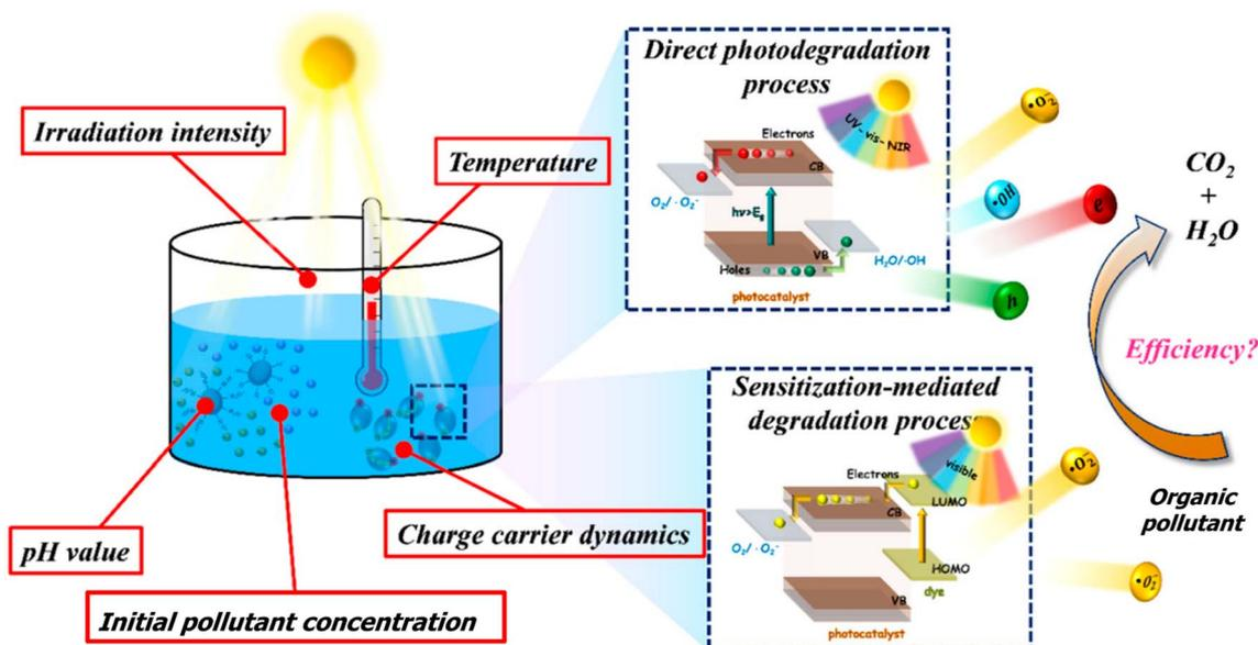
Fig. 10 Schematic shown of operational parameters affecting the photocatalytic degradation of organic pollutants.<sup>81</sup>
