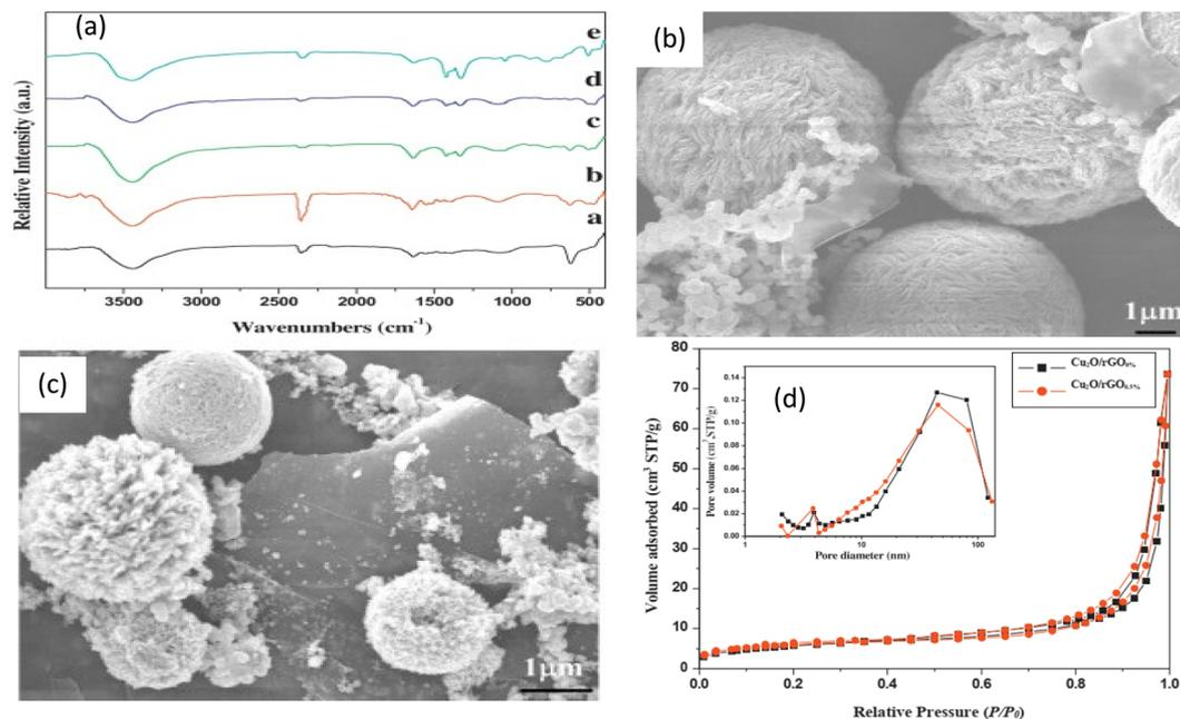
Fig. 2 (a) FT-IR spectra of as-prepared Cu<sub>2</sub>O/rGO<sub>x%</sub> samples with various wt% of rGO, (b and c) FESEM image of Cu<sub>2</sub>O/rGO 0.05, and 0.5% (wt%), respectively, and (d) N<sub>2</sub>-adsorption isotherms of Cu<sub>2</sub>O/rGO<sub>0%</sub> and Cu<sub>2</sub>O/rGO<sub>0.5%</sub> (wt) reprinted with permission from ref. 54. Copyright 2022 Elsevier.
