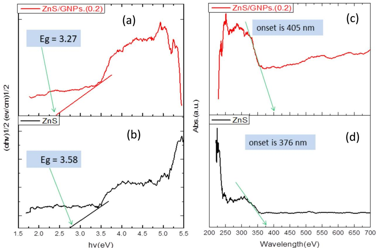
Fig. 6 Band gaps of ZnS/G NPs (a) and ZnS (b); and diffuse reflectance spectra of ZnS/G NPs (c) and ZnS (d), respectively.<sup>55</sup>
