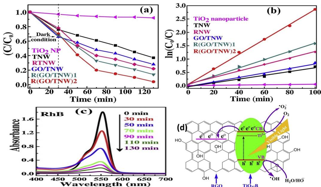
Fig. 9 (a) Plot of  $(C/C_0)$  versus time for degradation of RhB in the visible light, (b) kinetics of photodecomposition of the prepared samples, and (c) the absorption spectra of RhB under visible light irradiation catalyzed by  $\text{R}(\text{GO}/\text{TNW})_2$  composite, and (d) schematic diagram elucidating the mechanism of photocatalytic activity of  $\text{R}(\text{GO}/\text{TNW})_2$  reprinted with permission from ref. 78. Copyright 2022 Elsevier.
