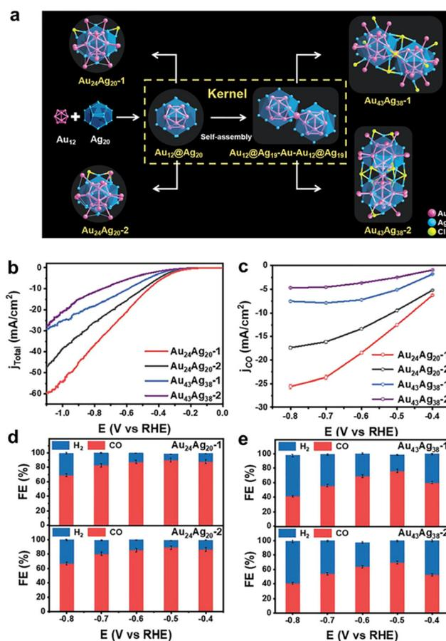
Fig. 13 (a) Structural anatomy of four nanoclusters. (b) LSV curves and (c) the corresponding CO partial current density of the  $\text{Au}_{24}\text{Ag}_{20}$  and  $\text{Au}_{43}\text{Ag}_{38}$  nanoclusters. Faradaic efficiency for  $\text{CO}_2\text{RR}$  products obtained on (d)  $\text{Au}_{24}\text{Ag}_{20}$  and (e)  $\text{Au}_{43}\text{Ag}_{38}$  nanoclusters. Copyright 2022, Royal Society of Chemistry.<sup>75</sup>
