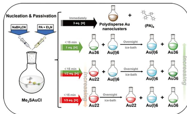
Fig. 6 Synthetic routes for Au<sub>36</sub>(PA)<sub>24</sub> with the different amounts of reducing agents in the synchronous nucleation and passivation strategy. Copyright 2020, Springer.<sup>47</sup>
