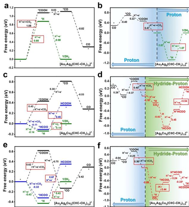
Fig. 10 Free energy of eCO<sub>2</sub>RR and HER on (a) and (b) intact and incomplete Au<sub>7</sub>Ag<sub>8</sub>, (c) and (d) Ag<sub>9</sub>Cu<sub>6</sub> and (e) and (f) Au<sub>2</sub>Ag<sub>8</sub>Cu<sub>5</sub>. Copyright 2022, Royal Society of Chemistry.<sup>95</sup>
