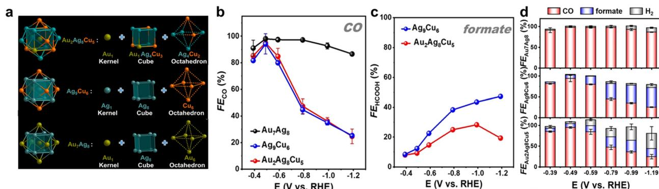
Fig. 9 (a) Structural anatomy of three nanoclusters. (b)  $\text{FE}_{\text{CO}}$  of three nanoclusters and (c)  $\text{FE}_{\text{formate}}$  of  $[\text{Ag}_9\text{Cu}_6(\text{C}\equiv\text{C}^t\text{Bu})_{12}]^+$ ,  $[\text{Au}_2\text{Ag}_8\text{Cu}_5(\text{C}\equiv\text{C}^t\text{Bu})_{12}]^+$ . (d) Product selectivity of three nanoclusters. Copyright 2022, Royal Society of Chemistry.<sup>95</sup>
