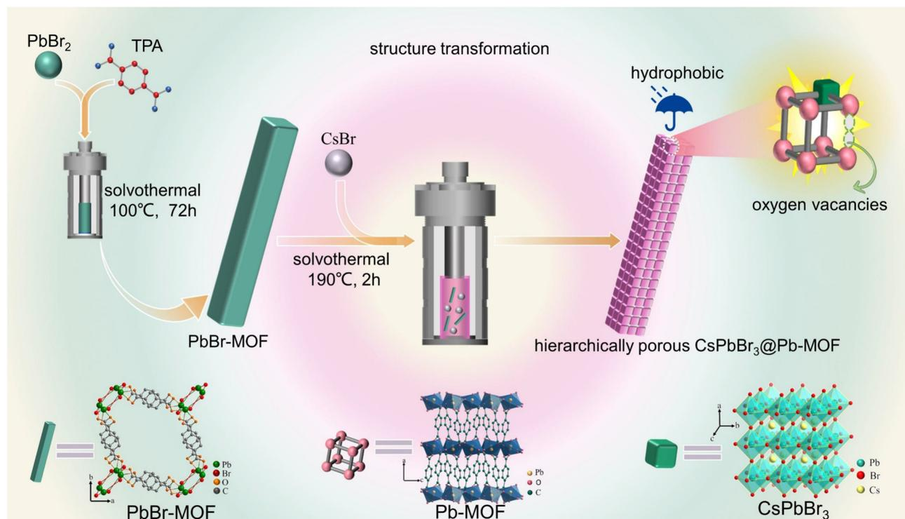
Fig. 1 A schematic diagram for the synthesis of CsPbBr<sub>3</sub>@Pb-MOF.
