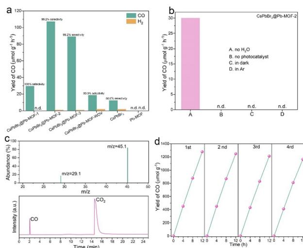
**Fig. 6** (a) Photoreduction CO<sub>2</sub> performances of the samples. (b) The photocatalytic performance of CsPbBr<sub>3</sub>@Pb-MOF-2 under different conditions. (c) The GC chromatogram and GC-mass result of an isotopic experiment using <sup>13</sup>CO<sub>2</sub>. (d) 48 h recycle photocatalytic CO<sub>2</sub> reduction using CsPbBr<sub>3</sub>@Pb-MOF-2.
