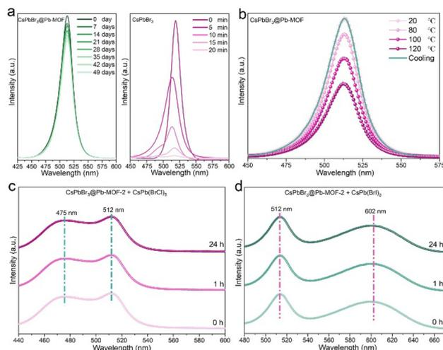
**Fig. 4** (a) PL intensity changes of CsPbBr<sub>3</sub>@Pb-MOF-2 and CsPbBr<sub>3</sub> with time. (b) The PL spectra of CsPbBr<sub>3</sub>@Pb-MOF-2 as a function of temperature. PL spectra of (c) CsPbBr<sub>3</sub>@Pb-MOF-2 and CsPb(BrCl)<sub>3</sub> and (d) CsPbBr<sub>3</sub>@Pb-MOF-2 and CsPb(BrI)<sub>3</sub> mixed powders at different time intervals.
