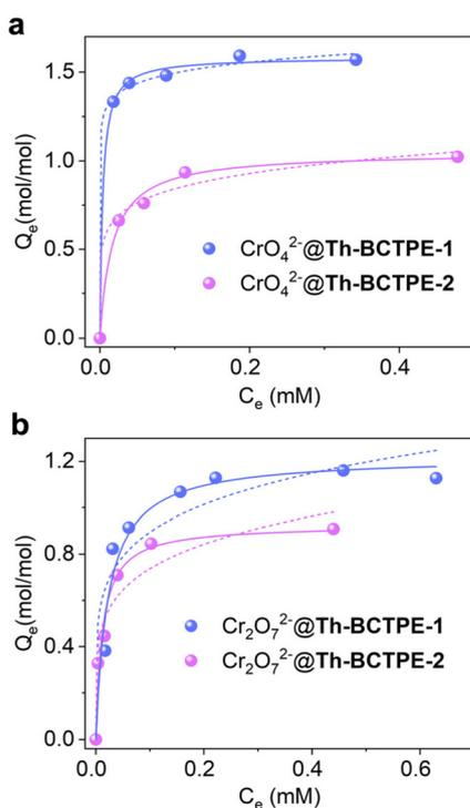
**Fig. 5** Adsorption isotherms of **Th-BCTPE-1** and **Th-BCTPE-2** for (a)  $\text{CrO}_4^{2-}$  and (b)  $\text{Cr}_2\text{O}_7^{2-}$  fitted with the Langmuir model (solid line) and the Freundlich model (dashed line).
