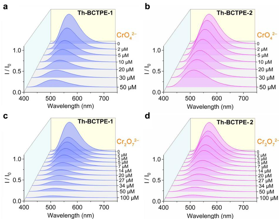
**Fig. 3** Normalized luminescence spectra of (a) Th-BCTPE-1 as a function of increasing  $\text{CrO}_4^{2-}$  concentration, (b) Th-BCTPE-2 as a function of increasing  $\text{CrO}_4^{2-}$  concentration, (c) Th-BCTPE-1 as a function of increasing  $\text{Cr}_2\text{O}_7^{2-}$  concentration, and (d) Th-BCTPE-2 as a function of increasing  $\text{Cr}_2\text{O}_7^{2-}$  concentration.
