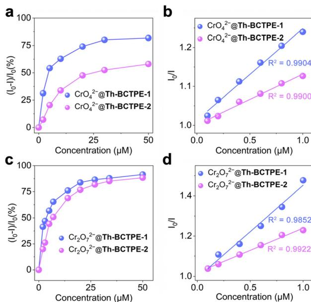
**Fig. 4** (a) The quenching rates of Th-BCTPE-1 and Th-BCTPE-2 as a function of  $\text{CrO}_4^{2-}$  concentration. (b) Stern–Volmer plots of luminescence quenching of Th-BCTPE-1 and Th-BCTPE-2 in  $\text{CrO}_4^{2-}$  solution. (c) The quenching rates of Th-BCTPE-1 and Th-BCTPE-2 as a function of  $\text{Cr}_2\text{O}_7^{2-}$  concentration. (d) Stern–Volmer plots of luminescence quenching of Th-BCTPE-1 and Th-BCTPE-2 in  $\text{Cr}_2\text{O}_7^{2-}$  solution.
