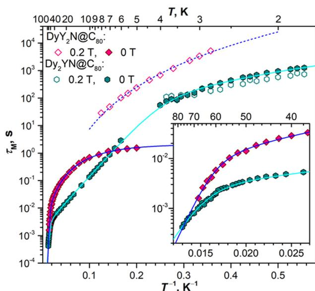
**Fig. 9** Magnetization relaxation times of DyY<sub>2</sub>N@C<sub>80</sub> and Dy<sub>2</sub>YN@C<sub>80</sub> determined by DC and AC magnetometry (open points, at 0.2 T; filled points, at zero field). Lines are fits with relaxation mechanisms discussed in the text. The inset shows enlargement of the high-temperature part.
