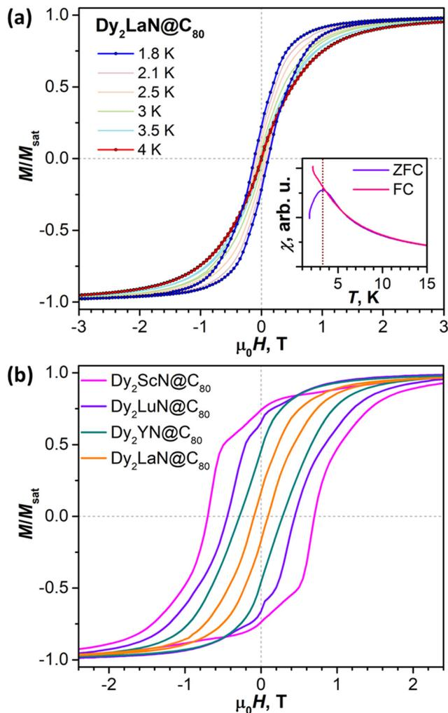
**Fig. 7** (a) Magnetic hysteresis measurements for  $\text{Dy}_2\text{LaN@C}_{80}$  (magnetic field sweep rate:  $2.9 \text{ mT s}^{-1}$ ); the inset shows determination of  $T_B$  from FC/ZFC measurements. (b) Comparison of the magnetic hysteresis shape for  $\text{Dy}_2\text{MN@C}_{80}$  EMFs ( $M = \text{Sc, Lu, Y, La}$ ) at 2 K (2.1 K for La); magnetic field sweep rate:  $2.9 \text{ mT s}^{-1}$  for all compounds.
