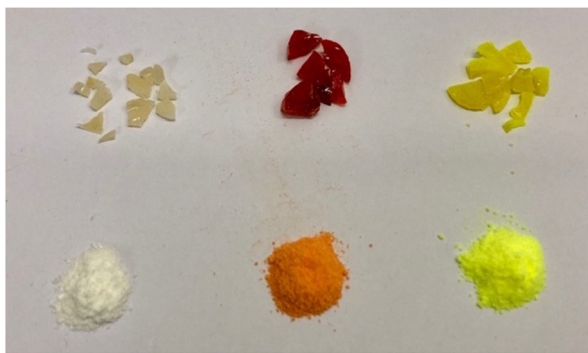
Fig. 2 ROCOP polymer samples; powdered products are shown below the corresponding melt-cast samples. From left to right, PA-CHO, AAQ-PA-CHO (0.2%), Nap-PA-CHO (0.2%).
