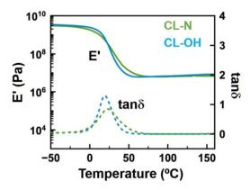
Fig. 2 Temperature-sweep rheology data for CL-N and CL-OH.
