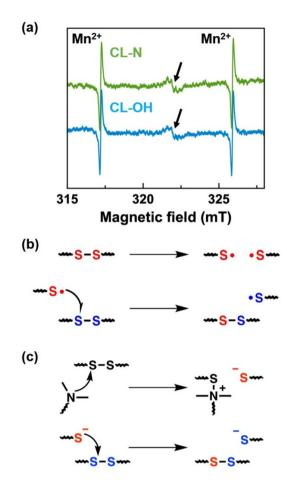
Fig. 5 (a) ESR spectroscopy data for CL-N and CL-OH measured at 160 °C. The arrows represent the signal from the sulfide radical, and the distinct outside signals were from Mn<sup>2+</sup> used for the magnetic field calibration. (b) The bond exchange mechanism of the disulfide bond via a radical-mediated mechanism and (c) a thiolate anion-mediated mechanism in the presence of tertiary amines.
