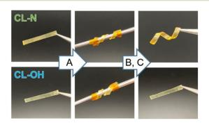
Fig. 4 Difference of reprocessability between CL-N and CL-OH during the process with A: fixing the sample with kapton tapes, B: heating in an oven (150 °C, 30 min), and C: cooling to 25 °C (room temperature).
