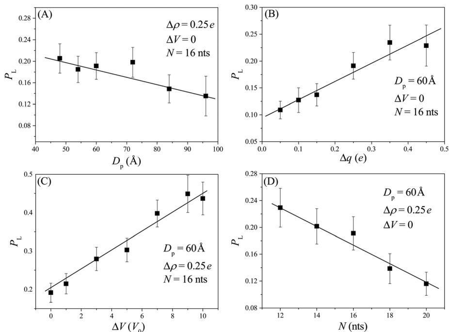
**Fig. 2** The successful landing probability  $P_L$  of the nanorobot as a function of pore–pore distance  $D_p$  (A), pore charge gradient  $\Delta q$  (B), external voltage  $\Delta V$  (C), and the leg length  $N$  (D). The lines serve as a visual guide. It should be noted that the data point at  $D_p = 96$  Å presented in panel (A) is an average of 40 samples due to the long computational time required.
