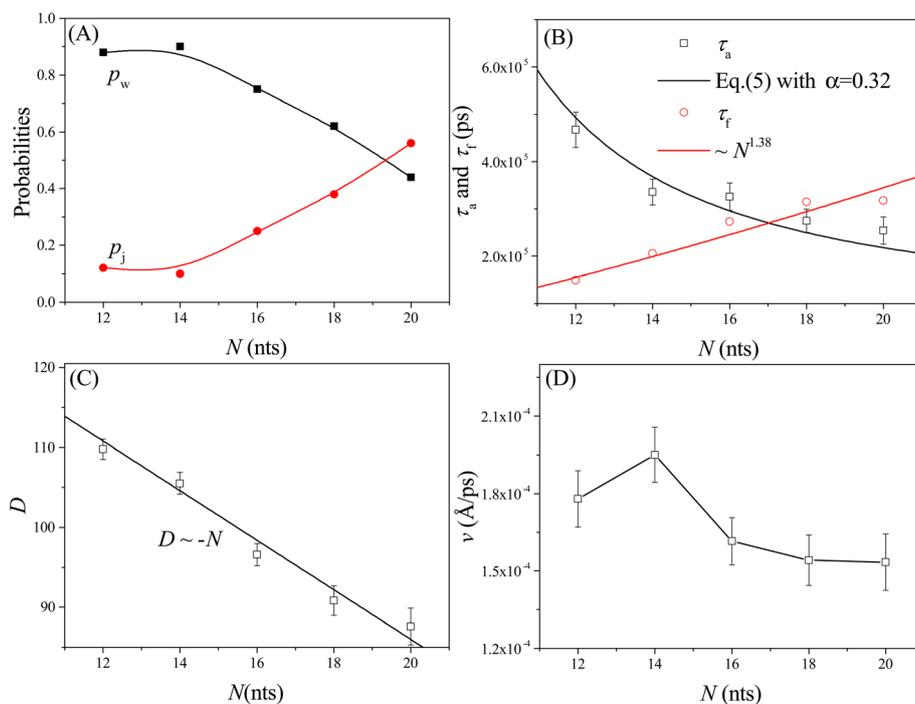
**Fig. 8** The leg length  $N$ -dependent walking and jumping probabilities  $p_w$  and  $p_j$  (A), conformational adjustment duration and forward-moving duration  $\tau_a$  and  $\tau_f$  (B), moving distance  $D$  of the nanorobot from the state F2 to the state F4 (C), and moving velocity  $v$  from all simulation samples (D). Here  $D_p = 60 \text{ \AA}$ ,  $\Delta q = 0.25e$ , and  $\Delta V = 0$ .
