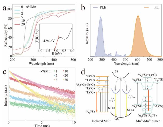
**Fig. 2** (a) Diffuse reflectance spectra of CCCP:*x*%Mn crystals and the plot of  $(F(R)h\nu)^2$  versus the light energy  $h\nu$  (inset). (b) Excitation and emission spectra of the CCCP:10%Mn crystals. (c) The fluorescence decay curve of the CCCP:*x*%Mn crystals ( $\lambda_{\text{ex}} = 290 \text{ nm}$ ,  $\lambda_{\text{em}} = 605 \text{ nm}$ ). (d) Schematic diagram for the photophysical processes in CCCP:Mn crystals.
