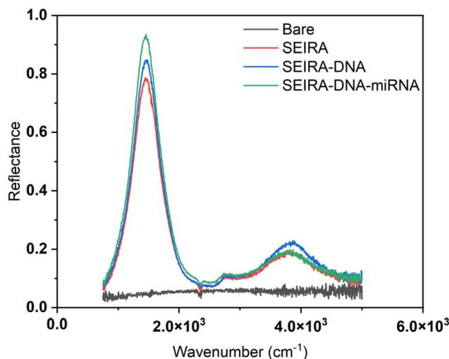
**Fig. 5** SEIRA enhancement. Reflectance measurements of a bare area without SEIRA, shown as black, an area with SEIRA structures when it was clean (red), after DNA binding (blue), and after miRNA binding (green).
