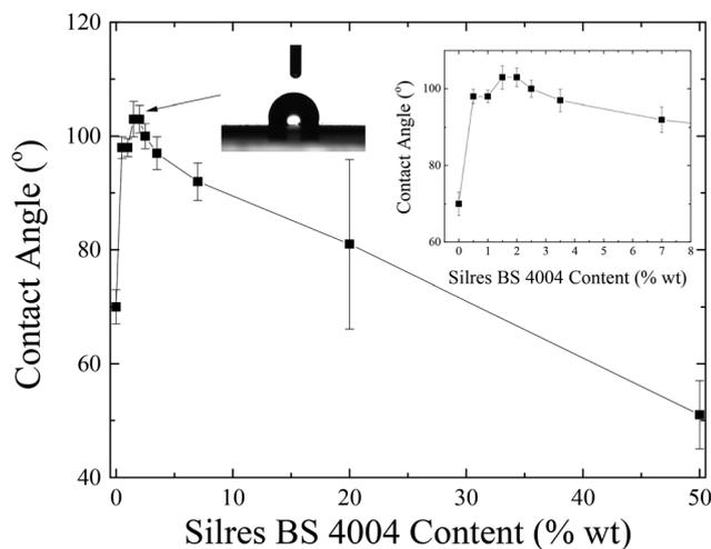
**Fig. 7** Equilibrium contact angles of water drops measured onto corona treated LDPE substrates coated with Silres BS 4004 as a function of Silres BS 4004 concentration in water. The insets show enlarged the low concentration regime as well as a representative photograph of a water drop on the surface coated with Silres BS 4004 at 2 wt% concentration, *i.e.*, for the surface that exhibits the maximum contact angle.
