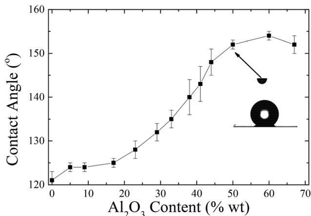
**Fig. 13** Equilibrium water contact angles measured for corona treated LDPE film surfaces coated utilizing aqueous dispersions containing Dynasylan SIVO (at 1 wt%) and PG003 alumina nanoparticles as a function of the concentration of the nanoparticles in the coating. A photograph of a water droplet is shown for a 50 wt% concentration of the nanoparticles.
