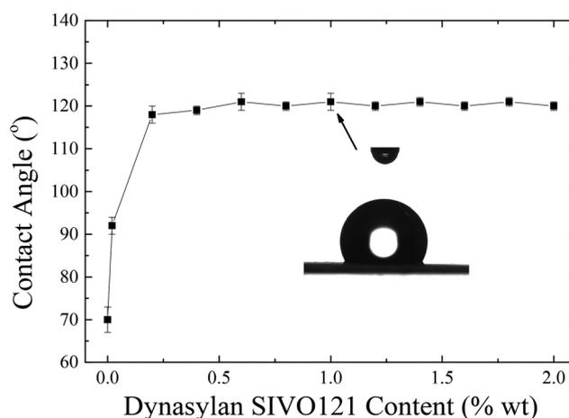
**Fig. 12** Equilibrium contact angles of water drops measured onto corona treated LDPE substrates coated with Dynasytan SIVO 121 films as a function of the Dynasytan concentration in water. The inset shows a photograph of a water drop on the surface coated with Dynasytan at 1 wt% concentration.
