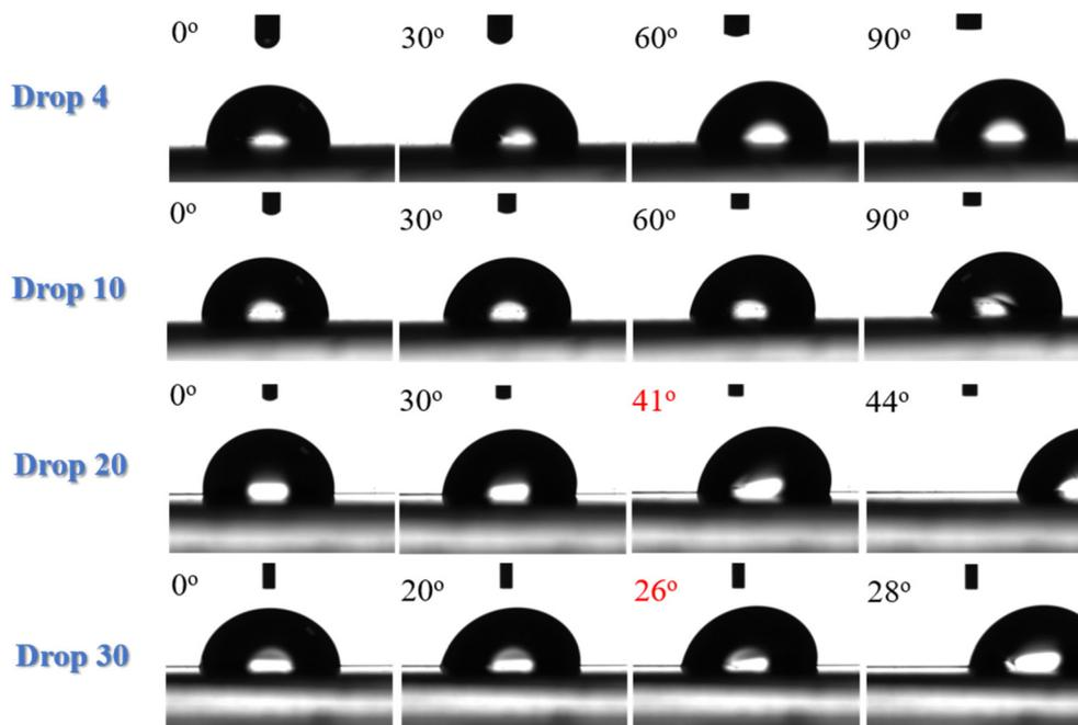
Fig. 2 Measurements of the roll off angles for water drops of 4, 10, 20 and 30  $\mu\text{L}$  (from top row to bottom) on a neat LDPE film. The red numbers on the up left corner shows the roll off angle for the 20  $\mu\text{L}$  and 30  $\mu\text{L}$  droplets, which are  $41^\circ$  and  $26^\circ$ , respectively.
