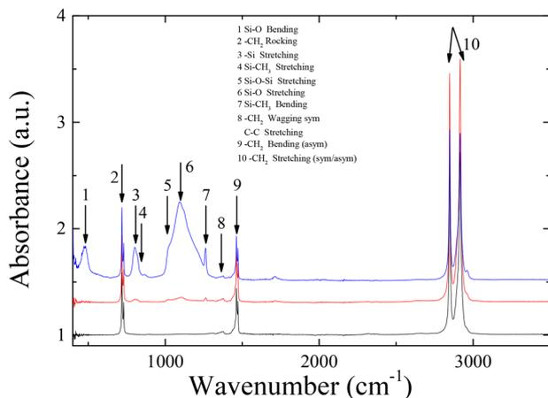
**Fig. 6** ATR-FTIR spectra of corona treated LDPE film (black), corona treated LDPE coated with Silres of 2 wt% concentration in water (red) and corona treated LDPE coated with the nanocomposite Silres/ZL 77%/23% (blue).
