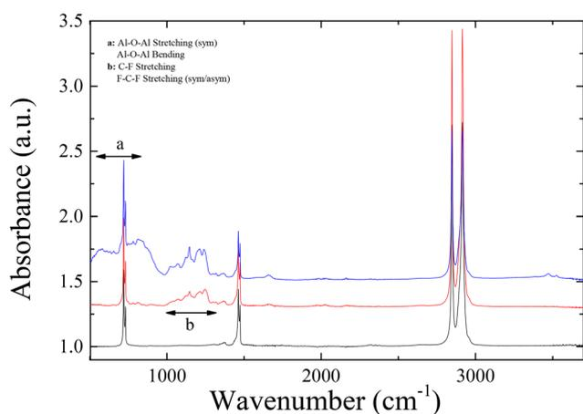
**Fig. 11** ATR-FTIR spectra of corona treated LDPE (black), corona treated LDPE coated with Dynasytan SIVO 121 of 1 wt% concentration in water (red) and corona treated LDPE coated with the nanocomposite Dynasytan SIVO 121/PG003 66%/34% (blue).
