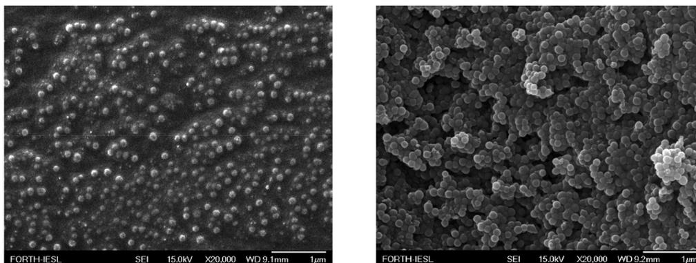
**Fig. 10** SEM images of LDPE films, after the deposition of a nanocomposite coating consisting of (left) 67 wt% Silres BS 4004 and 33 wt% ZL nanoparticles and (right) 33 wt% Silres BS 4004 and 67 wt% ZL nanoparticles.
