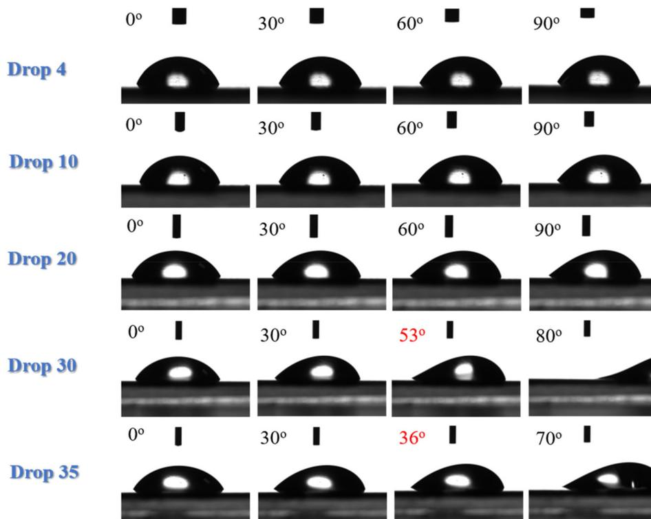
Fig. 4 Measurements of the roll off angles for water droplets of 4, 10, 20, 30 and 35  $\mu\text{L}$  (from top row to bottom) on a corona treated LDPE film. The red numbers on the up left corner shows the roll off angle for the 30  $\mu\text{L}$  and 35  $\mu\text{L}$  droplets, which are 53° and 36°, respectively.
