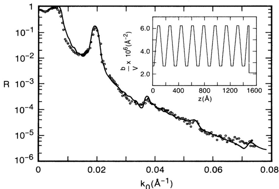
**Fig. 6** The specular neutron reflectivity as a function of neutron wavevector  $k_{z0}$  ( $Q = Q_z = 2k_{z0}$ ) for a P(S-*b*-D-MMA) diblock copolymer film on a Si substrate after annealing for 24 h at 170 °C. The inset shows the SLD profile from which a reflectivity was calculated (solid line) and fit to the data (open circles). (After Fig. 1 of Anastasiadis *et al.*<sup>13</sup>).
