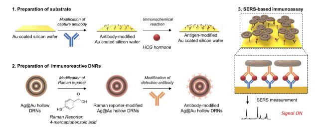
Fig. 5 Schematic illustration of the strategy of the SERS-based immunoassay. Antibody-modified Aq-Au DRNs are distributed onto human chorionic gonadotropin (HCG) bound Au-coated silicon wafers to form a sandwich formation measured by SERS.
