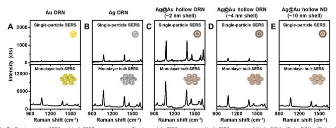
Fig. 3 Single-particle SERS and bulk SERS measurements. Single-particle SERS spectra and bulk SERS spectra of (A) Au DRNs, (B) Ag DRNs, (C) Ag@Au hollow DRNs (the thickness of Ag-Au shell: ~2 nm), (D) Ag@Au hollow DRNs (the thickness of Ag-Au shell: ~4 nm), and (E) Ag@Au hollow nanodisks (the thickness of Ag-Au shell:  $\sim 10$  nm).
