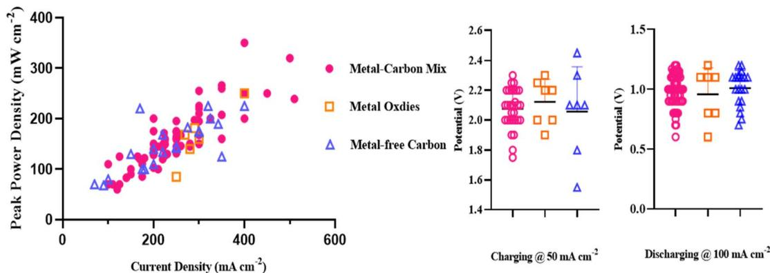
Fig. 23 Performance of different type of catalysts in the zinc-air battery according to reports.<sup>91,100,105,106,128,130,131,133–135,141,144,148,187,189,192,194,198,212,214,216,225,226,240,242,246,248,253–255,257,258,263,267,287,289,290,295,308,314,322,329–385</sup>
