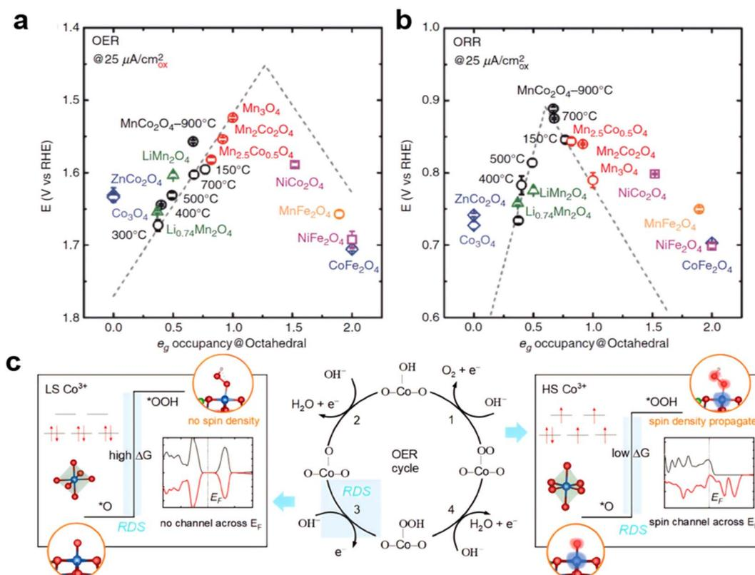
Fig. 8 (a) and (b) Volcano relationship between e<sub>g</sub> filling and OER/ORR performance. (reproduced from ref. 175 with permission. Copyright © 2017 Wiley-VCH). (c) High and low spin of Co and OER RDS. (Reproduced from ref. 178 with permission. Copyright © 2021 Wiley-VCH).
