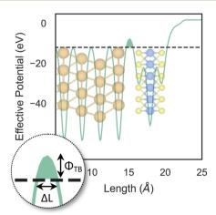
Fig. 6 Effective potential across the interface of the pristine  $Au/MoS_2$  structure. The potential was projected in the direction of the interface. Highlighted in the figure are the tunnelling barrier height ( $\Phi_{TB}$ ) and the barrier width ( $\Delta L$ ).
