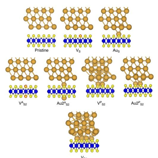
Fig. 2 Optimized geometries with DFT of selected Au/MoS<sub>2</sub> interfaces considered in this work. The pictures were taken in the vicinity of the contact area between the two materials. Interfaces  $V_{S2}^P$  and  $V_{S4}$  refer to MoS<sub>2</sub> with clusters of two and four S vacancies, although following geometry optimization such clusters were fully filled by Au atoms migrating from the above electrode.
