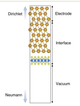
Fig. 1 Representative example of the Au/MoS<sub>2</sub> interface, modelled with the Green's function surface approach. The system can be divided into three parts: (1) the electrode (to which Dirichlet boundary conditions were applied), (2) the central part, consisting of 6 atomic layers of Au coupled with single-layer MoS2, and (3) the vacuum region, to which Neumann boundary conditions were applied.
