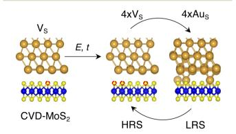
Fig. 8 Illustration of the proposed resistive switching mechanism and the possible  $Au/MoS_2$  interfaces involved. Here, we propose the electric field (*E*) and/or temperature (*t*) as key quantities to generate extra S vacancies and to force the migration of Au atoms from (to) the metal electrode.
