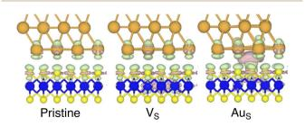
Fig. 4 Electron density difference (EDD) maps of the pristine,  $V_{S}$ , and  $Au_{S}$  interfaces in the vicinity of the contact area. Green colour corresponds to electron loss, whereas mauve colour to electron enrichment. The isovalue was set to 0.002 eV  ${\rm \mathring{A}}^{-3}$ .
