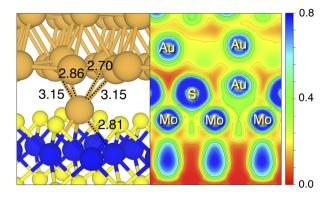
Fig. 3 Optimized geometry of the  $Au_S$  interface (left image), in the proximity of the contact area. Relevant Au-Mo and Au-Au bond lengths (in angstrom) are shown. Contour plot of the ELF for the  $Au_S$  interface (right image) in the proximity of the contact area. The color scheme is RGB, and red corresponds to ELF = 0, whereas blue to ELF = 0.8.
