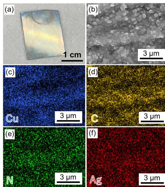
Fig. 4 (a) A photo of the AgNPs@ $\text{Cu}_2(\text{BPYDC})_2$ -on- $\text{Cu}_2(\text{BPDC})_2$  thin film. (b) SEM and (c–f) EDS mapping images of the AgNPs@ $\text{Cu}_2(\text{BPYDC})_2$ -on- $\text{Cu}_2(\text{BPDC})_2$  thin film.
