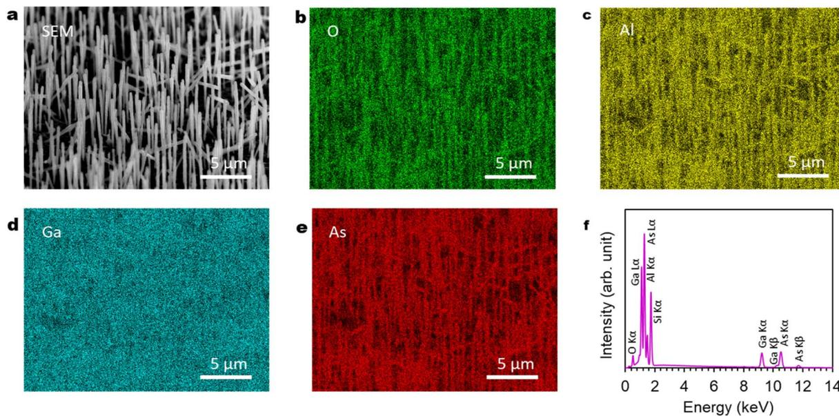
Fig. 7 SEM and EDS results for GaAs/Al<sub>0.8</sub>Ga<sub>0.2</sub>As core-shell nanowires: (a) 45°-tilted SEM image. (b)–(e) EDS elemental mapping images of O, Al, Ga, As. (f) EDS spectra from the imaging area. The images were obtained with an acceleration voltage of 25 kV.
