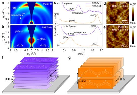
Fig. 2 Thin-film microstructures. (a) and (b) 2D GIWAXS patterns of PBBT-H (a) and PBBT-Me (b). (c) In-plane and out-of-plane GIWAXS line cuts of PBBT-H and PBBT-Me thin films. (d) and (e) AFM height images of PBBT-H (d) and PBBT-Me (e). The root mean square (RMS) surface roughness is also reported. (f) and (g) Schematic of the PBBT-H and PBBT-Me chains packing.
