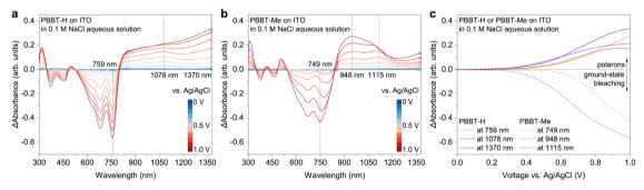
Fig. 3 Differential spectroelectrochemistry. (a) and (b) Differential absorption spectra of PBBT-H (a) and PBBT-Me (b). (c) Differential absorption spectra of PBBT-H (c) and PBBT-Me (d) at select wavelengths. In all these spectroelectrochemistry measurements, 0.1 M NaCl aqueous solution was used as the electrolyte, Ag/AgCl electrode was grounded, and the voltage was applied to the polymer films scanning between 0 V and 1.0 V versus Ag/AgCl electrode.
