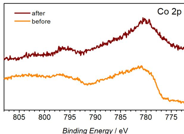
**Fig. 5** High-resolution Co 2p XP spectra of the **Co-TMBT-MOF/NF** electrodes before and after the 20 h OER tests in 1 M KOH at 20 mA cm<sup>-2</sup> and 23 ± 2 °C.
