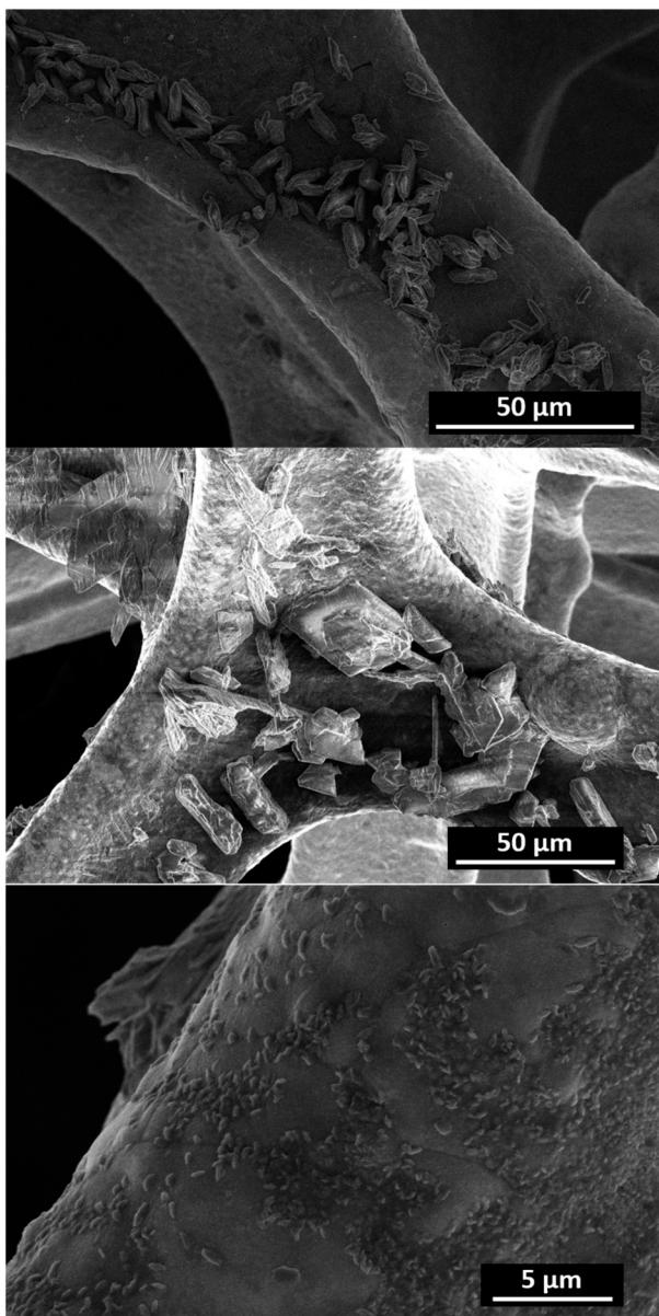
**Fig. 4** SEM images of **Co-TMBT-MOF/NF** before (top) and after the 20 h (centre and bottom) OER tests in 1 M KOH at 20 mA cm<sup>-2</sup> and 23 ± 2 °C.
