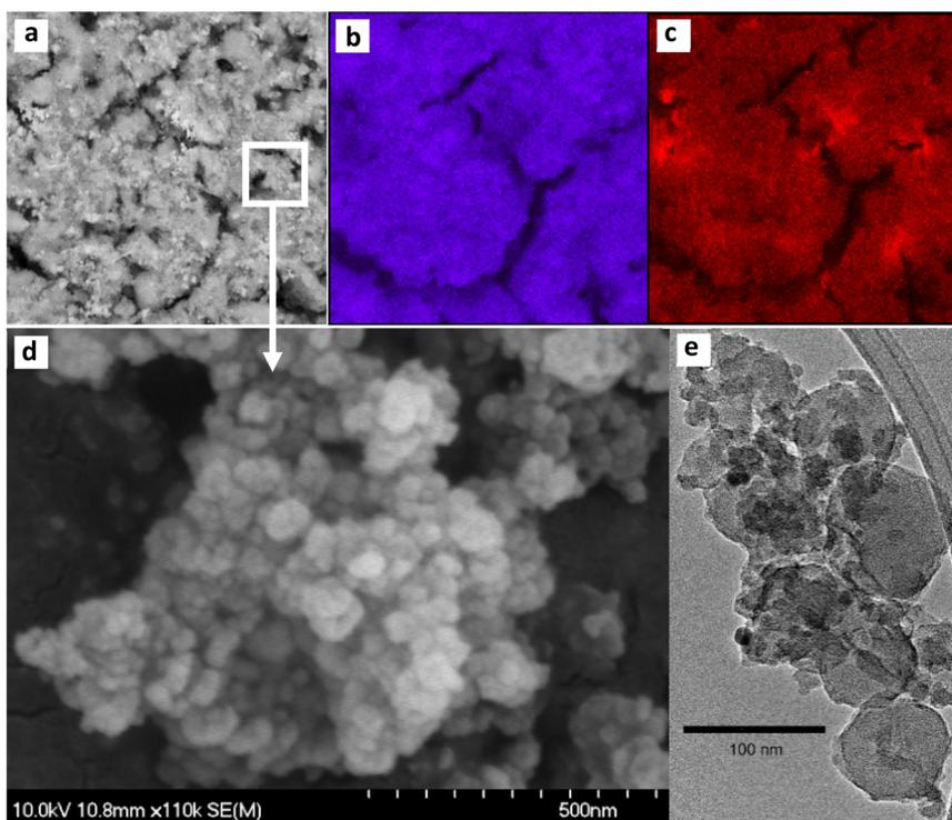
**Fig. 7** SEM micrographs of Ag/U(0.75)T sample: a) SEM image of a wide region of the solid; b) mapping of silver by EDS in the selected region; c) mapping of zirconium by EDS in the selected region; d) high magnification image by FE-SEM; e) TEM image.
