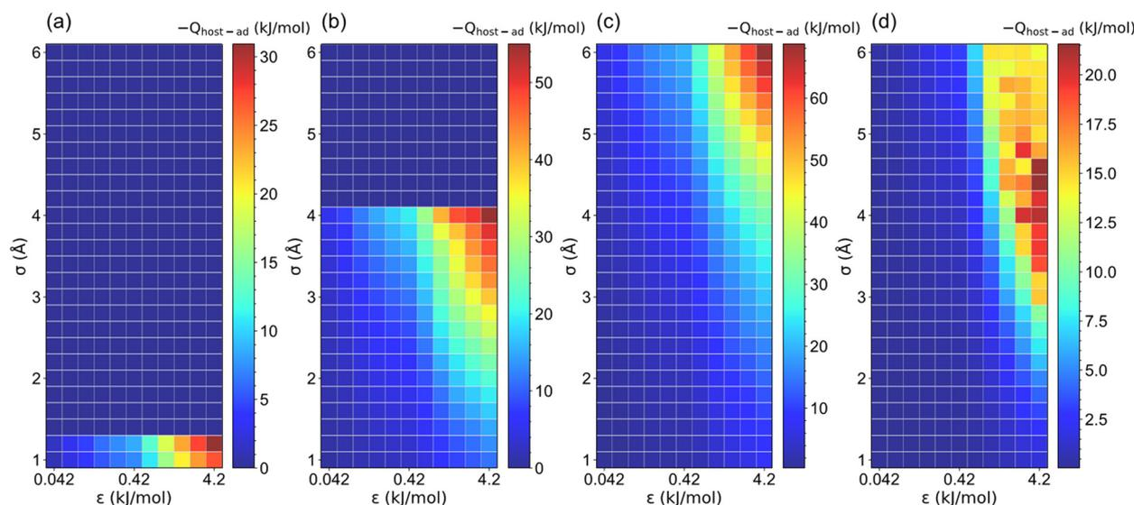
Fig. 8 The host-adsorbate interaction ( $Q_{\text{host-ad}}$ ) between pseudo material and ethanol under various LJ parameters ( $\sigma$  and  $\varepsilon$ ) for (a)  $l = 5$ , (b)  $l = 7.5$ , (c)  $l = 10$  and (d)  $l = 35 \text{ Å}$  structures.
