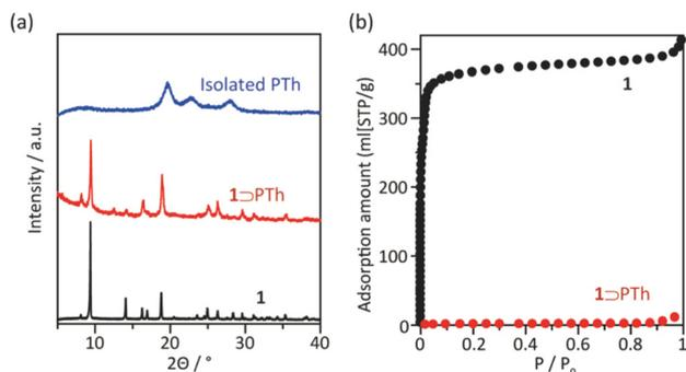
**Fig. 3** (a) XRPD patterns of **1**, **1**  $\supset$  PTh, and PTh liberated from **1**. (b)  $N_2$  adsorption isotherms of **1** and **1**  $\supset$  PTh at 77 K (**1**;  $S_{\text{BET}} = 1447 \text{ m}^2 \text{ g}^{-1}$ , **1**  $\supset$  PTh;  $S_{\text{BET}} = 4 \text{ m}^2 \text{ g}^{-1}$ ).
