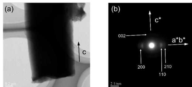
**Fig. 5** (a) TEM image and (b) selected area electron diffraction patterns of PTh from **1**.
