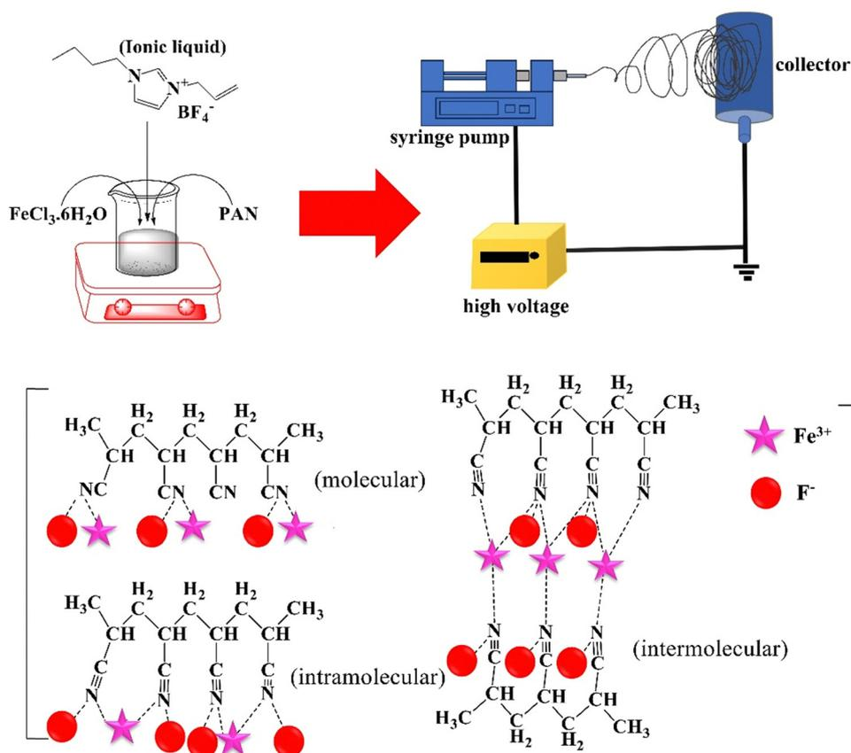
Fig. 2 Improved piezoelectricity of PAN NFs by their incorporation with 1-allyl-3-butylimidazolium tetrafluoroborate and  $\text{FeCl}_3$  (adapted from ref. 99 with permission from John Wiley and Sons).
