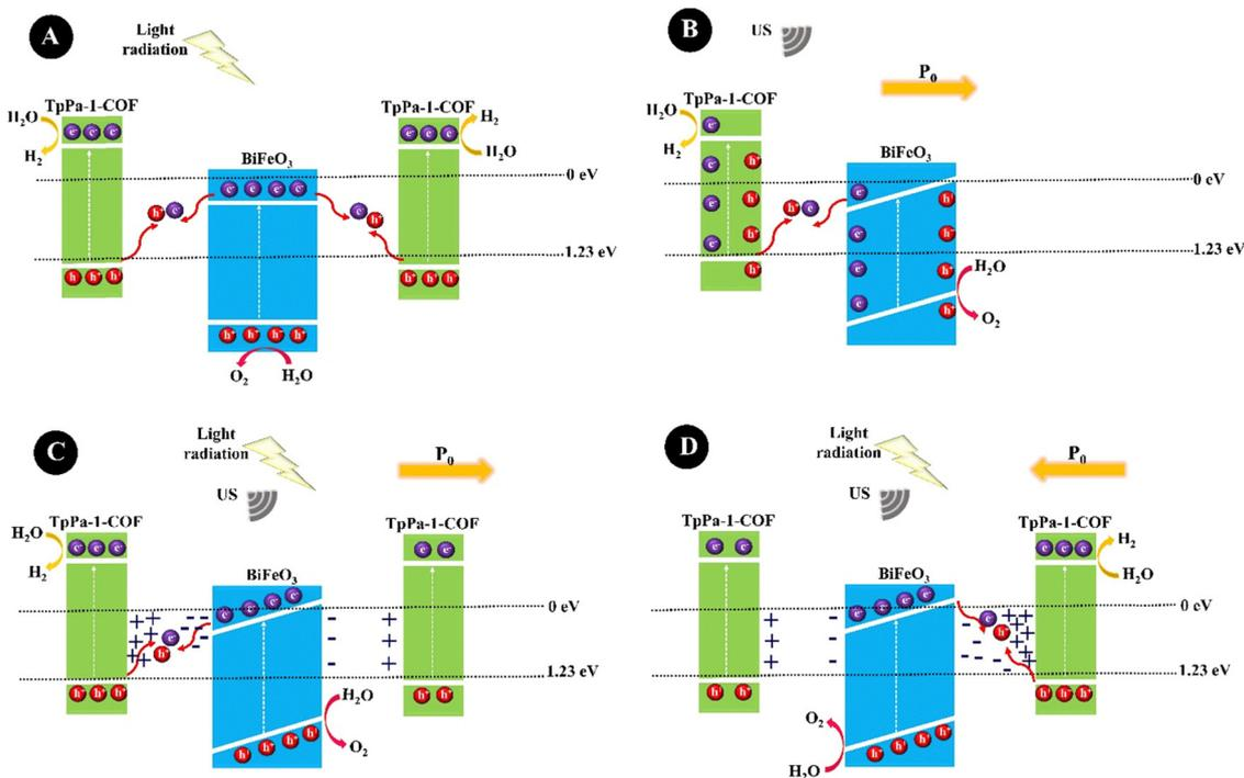
Fig. 4 The representative diagrams of photocatalysis (A), piezocatalysis (B), and piezo/photocatalysis (C) and (D) for  $\text{BiFeO}_3@$ TpPa-1-COF (adapted from ref. 162 with permission from John Wiley and Sons).
