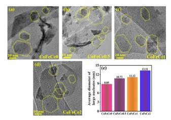
Fig. 5 (a)-(d) HRTEM images of different Ce-doped CoFe LDHs showing large nucleates (dotted vellow line), and (e) bar graph showing the trend in the average diameter of large nucleates in different LDHs
