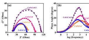
Fig. 8 (a) Nyquist plots, and (b) Bode plots at a bias potential of 1.54 V vs RHE in the frequency range from  $10^5$  to  $10^{-1}$  s<sup>-1</sup> with 0.005 V amplitude for different LDHs. The experimental results are represented by discrete points and equivalent circuit fitted results are represented by solid lines.
