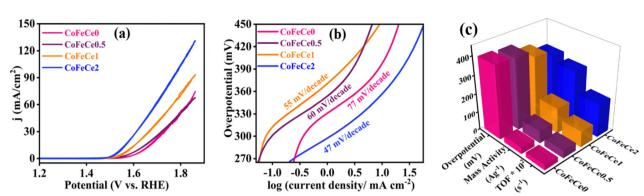
Fig. 6 Electrochemical results of LDHs. (a) CVs at a scan rate of 5 mV s $^{-1}$ , (b) Tafel plots of Ce-doped CoFe LDHs during water oxidation and (c) overpotentials, mass activities, and TOFs of the Ce-doped CoFe LDHs during water oxidation. Overpotentials were measured at 10 mA cm $^{-2}$  current density. Mass activities and TOFs were calculated at 350 mV overpotential.
