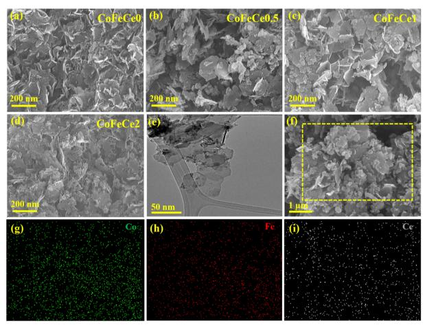
Fig. 2 Morphological characterization of Ce-doped CoFe-LDHs: (a) – (d) SEM image, (e) a low-resolution TEM micrograph of CoFeCe2 LDH, and (f) SEM image of CoFeCe2 LDH taken for elemental mapping. Elemental mapping for (g) Co, (h) Fe and (i) Ce from the selected area of the SEM image as shown in (f)
