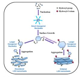
Schematic of the crystallization mechanism for LDH Scheme 2
