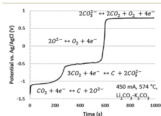
Fig. 13 Chrono-potentiometric plots for anodic oxidation of the electro-deposited carbon in  $\text{Li}_2\text{CO}_3$ - $\text{K}_2\text{CO}_3$  at  $574$  °C, reproduced from ref. 41 with open-access permission from the Royal Society of Chemistry, copyright 2014.
