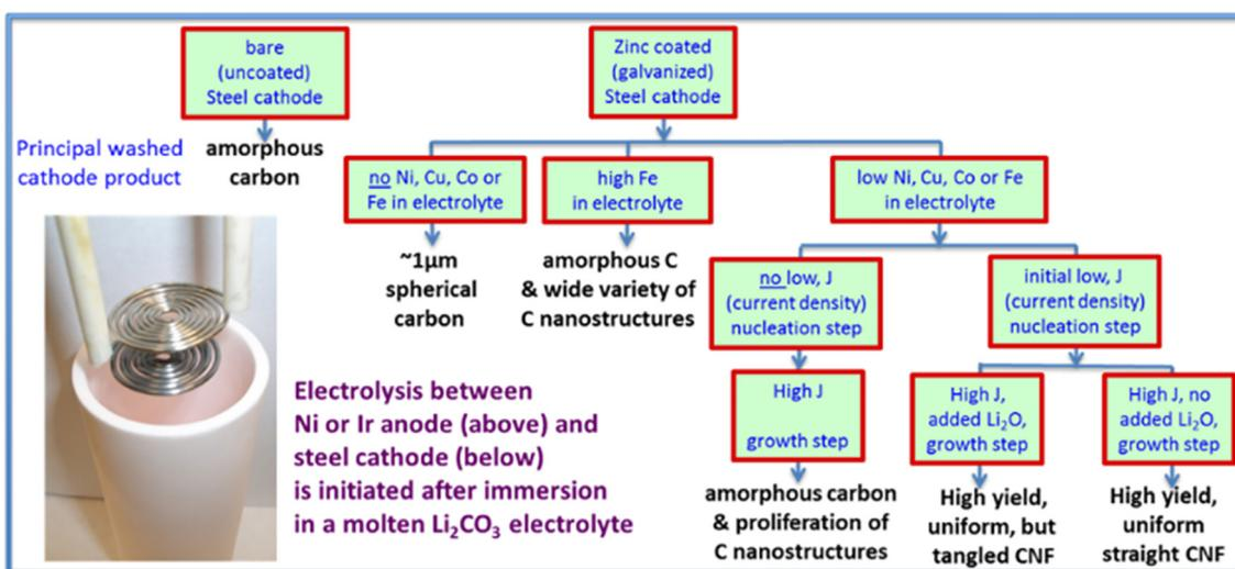
Fig. 8 Molten carbonate electrolysis pathways converting  $\text{CO}_2$  leading to high yield, uniform CNF product.<sup>92</sup>
