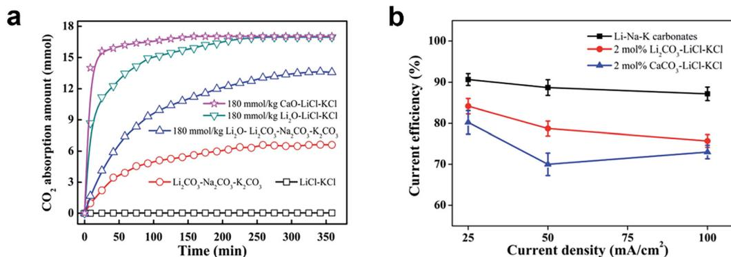
Fig. 6 (a) CO<sub>2</sub> absorption curves in different molten salts at 450 °C with the CO<sub>2</sub> partial pressure of 50 kPa; (b) current efficiency for galvanostatic electrolysis in different molten salts under CO<sub>2</sub> atmosphere at 450 °C.<sup>76</sup>
