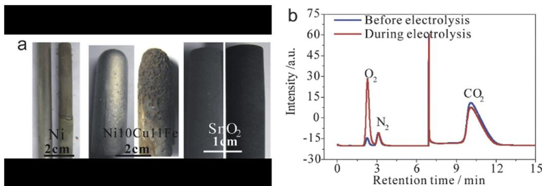
Fig. 10 (a) Digital photos of Ni,  $\text{Ni}_{10}\text{Cu}_{11}\text{Fe}$  and  $\text{SnO}_2$  electrodes before and after serving as the anode; (b) gas chromatograms of the outlet gas before and during electrolysis using the  $\text{SnO}_2$  anode.<sup>35</sup>
