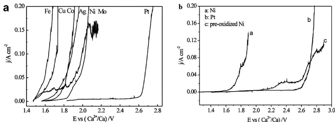
Fig. 11 (a) Polarization curves of metals in molten  $\text{CaCl}_2 - 2.5 \text{ mol\% CaO}$  at  $850 \text{ }^\circ\text{C}$  (potential scan rate,  $2 \text{ mV s}^{-1}$ ); (b) polarization curves of Ni, Pt and pre-oxidized Ni in molten  $\text{CaCl}_2$  at  $850 \text{ }^\circ\text{C}$  (potential scan rate,  $2 \text{ mV s}^{-1}$ ).<sup>103</sup>
