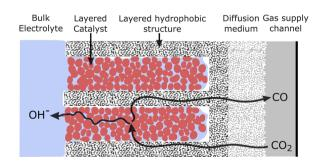
Fig. 8 Cross section of a cathode geometry with alternating layers of gasconducting hydrophobic material and catalyst nanoparticles. The layering geometry would extend the liquid-gas interface, providing a short liquid diffusion length to all catalyst nanoparticles.
