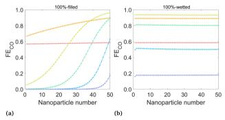
Fig. 6 Mean FE<sub>CO</sub> at the surface of each nanoparticle for (a) the 100%filled case and (b) the 100%-wetted case, at various applied potentials. Nanoparticles are numbered starting at 1 for the left-most (deepest) particle. (Legend same as Fig. 5)
