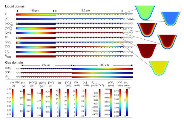
Potential, concentrations, and partial pressures for the 50%-filled case with a cathode potential of -1.1 V vs. RHE and a 0.1 M KHCO<sub>3</sub> electrolyte.
