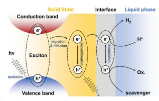
Fig. 1 Schematic diagram of organic semiconductor photocatalytic HER.
