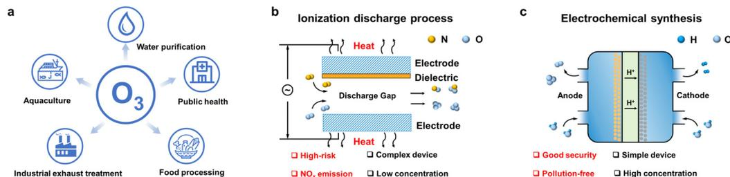
**Scheme 1** Applications and preparation methods of ozone. (a) Applications of ozone in various industries. (b) Ozone preparation through the ionization discharge process. (c) Ozone preparation by the electrochemical oxidation of water.
