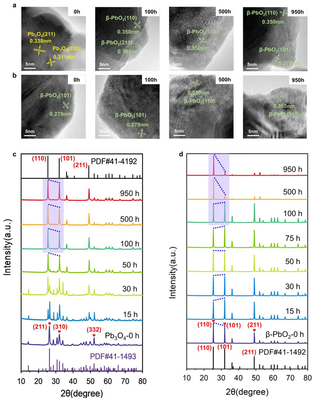
Fig. 2 Structural characterization of  $\text{Pb}_3\text{O}_4$  and  $\beta\text{-PbO}_2$  in MEA under different EOP durations. (a and b) HRTEM images and (c and d) *ex situ* XRD patterns of  $\text{Pb}_3\text{O}_4$  and  $\beta\text{-PbO}_2$  before and after EOP treatment in EOP electrolyzer at a high current of  $1 \text{ A cm}^{-2}$ .
