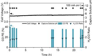
Fig. 4 Long-term operation of DCE over 23 hours with CO FE, H<sub>2</sub>/CO ratio, full cell voltage, and capture solution pH noted. Experiment conducted at a constant current density of 100 mA cm<sup>-2</sup> with a 1 cm<sup>2</sup> active area. Schematic and picture of the experimental set-up are provided in the ESI† (Fig. S10A and B).
