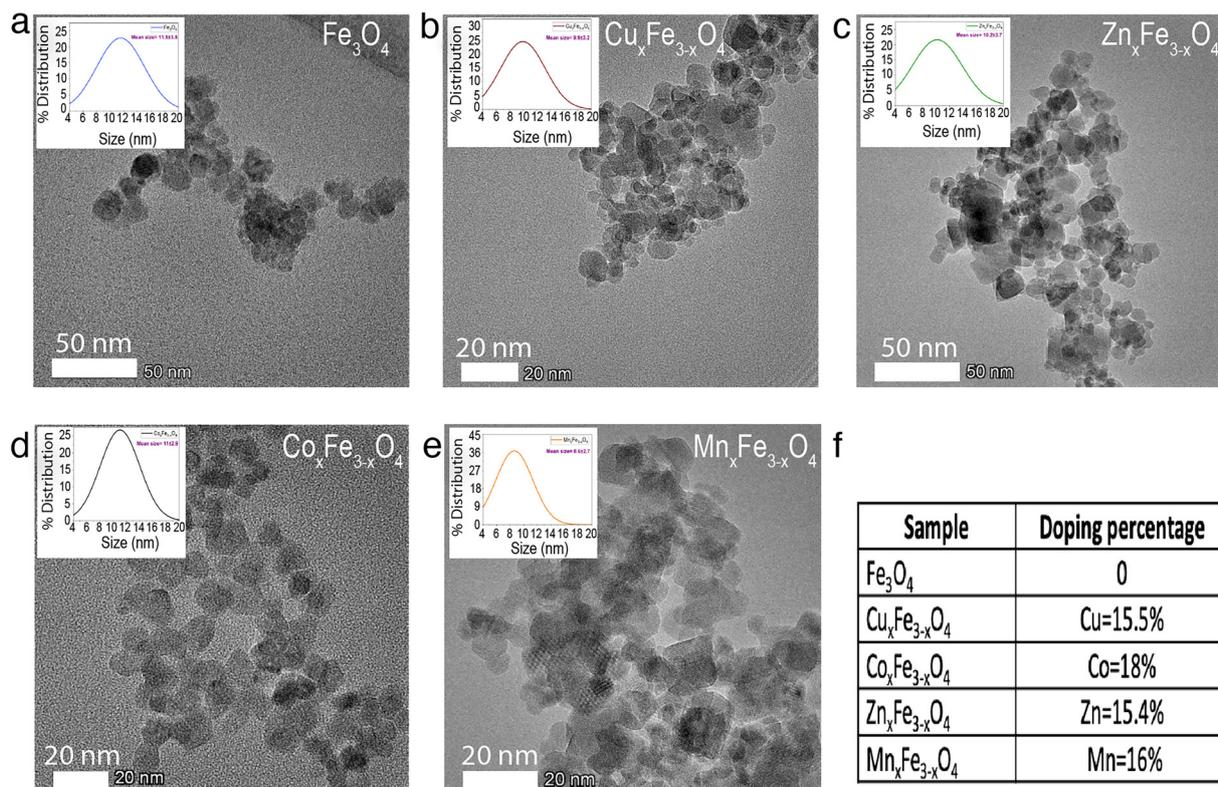
Fig. 2 TEM images showing the morphology and particle size distribution (shown in inset) of (a)  $\text{Fe}_3\text{O}_4$  (b)  $\text{Cu}_x\text{Fe}_{3-x}\text{O}_4$  (c)  $\text{Co}_x\text{Fe}_{3-x}\text{O}_4$  (d)  $\text{Zn}_x\text{Fe}_{3-x}\text{O}_4$  (e)  $\text{Mn}_x\text{Fe}_{3-x}\text{O}_4$ , (f) dopant concentration in ferrites as measured by ICP-MS.
