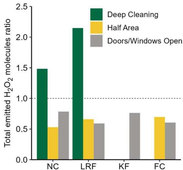
Fig. 5 Ratio of total emitted  $\text{H}_2\text{O}_2$  molecules under the cleaning conditions investigated (deep cleaning, half area, and door/windows open) to the standard controlled cleaning condition.
