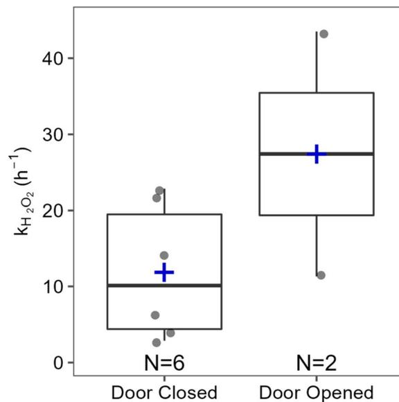
Fig. 4 Statistics of  $k_{\text{H}_2\text{O}_2}$  for regular cleaning of the near counter under different ventilation conditions. The box and whisker plots show the median (line), mean (blue marker), first and third quartiles (box), and minima and maxima (whiskers). The number under each box and whisker plot indicates the number of cleaning events for that condition.
