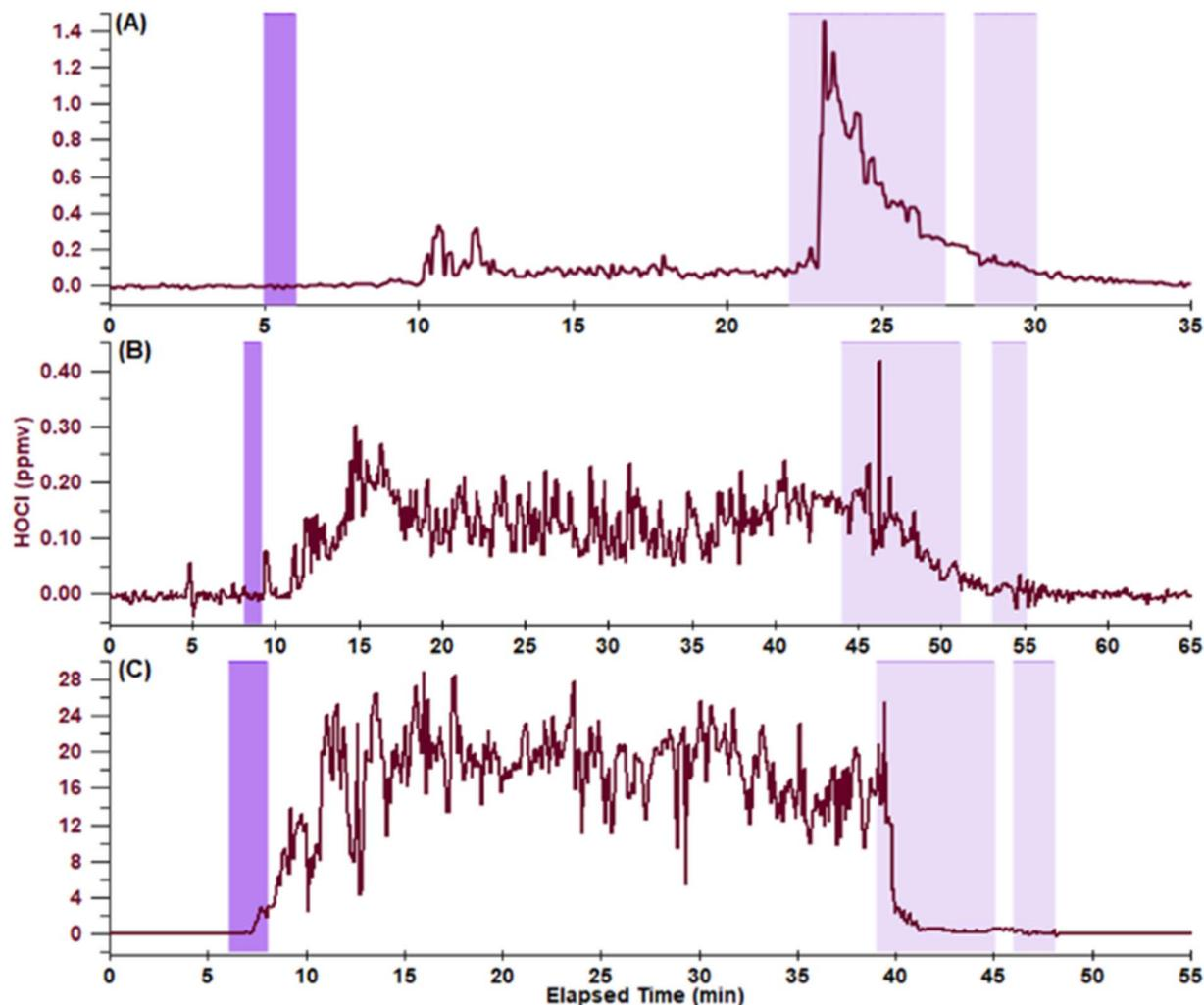
Fig. 1 Representative time series of HOCl mixing ratios during stationary measurements of bathtub cleaning events with the inlet at (A) near-ceiling, (B) mid-room, and (C) near-tub positions. Time intervals during which the cleaner was sprayed onto the bathtub surface are denoted by dark purple, and subsequent time intervals for scrubbing and rinsing of the bathtub (always in that sequence) are denoted by light purple.
